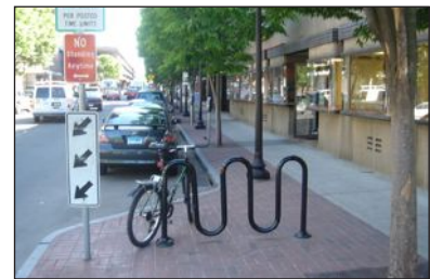
Bump-outs with bike racks, downtown New Haven
