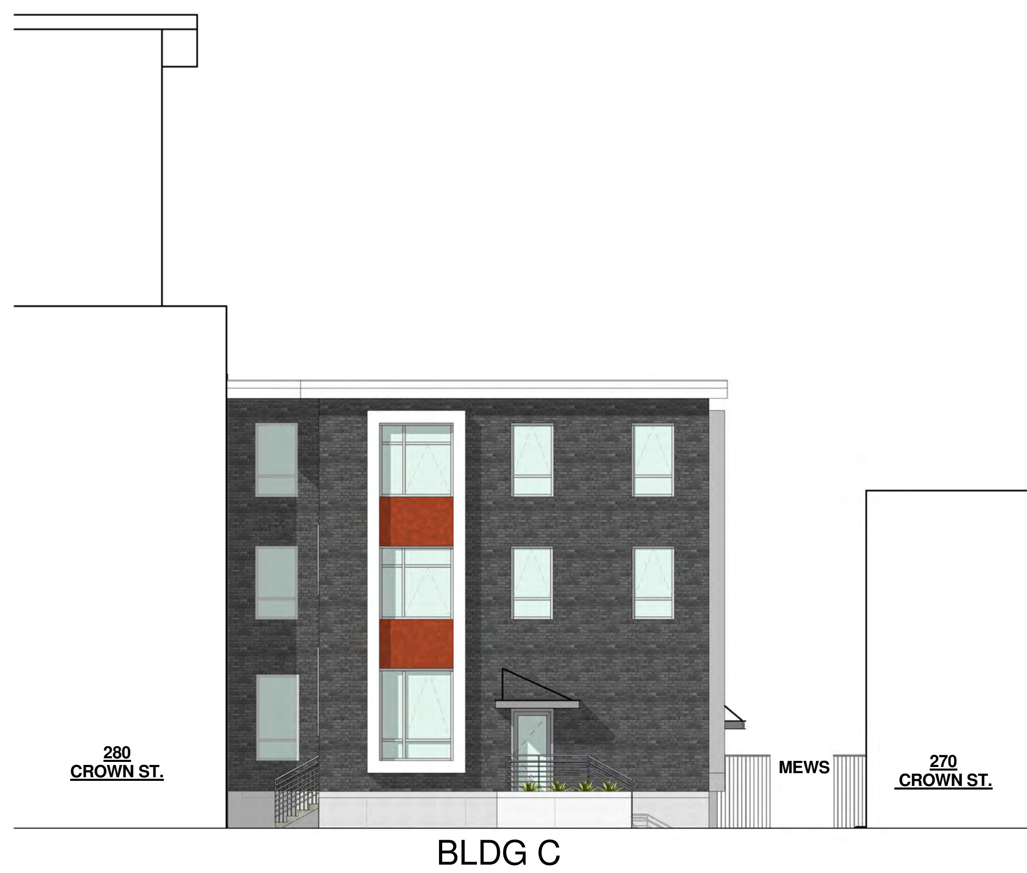
③ BUILDING C - SOUTH ELEVATION 1/8" = 1'-0"
