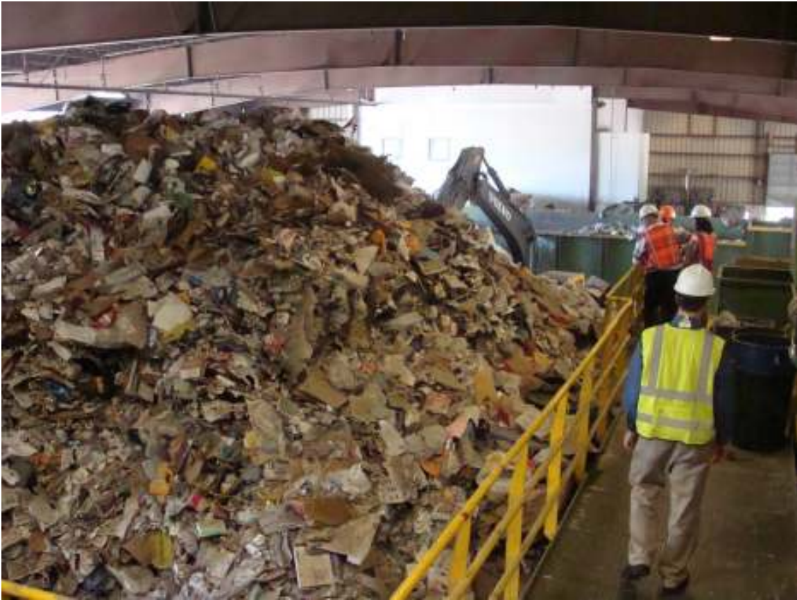
Picture 2: Recyclables are loaded into the sorting apparatus by machine.
