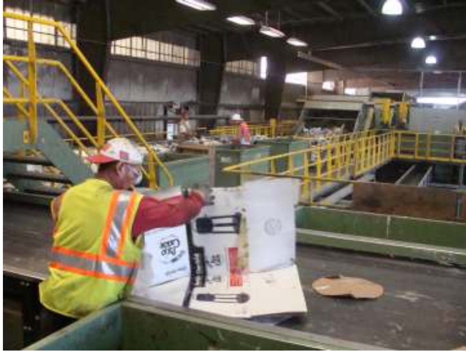
Picture 5: Some manual sorting increases the quality of the final products and removes items that may jam or break the machine.
