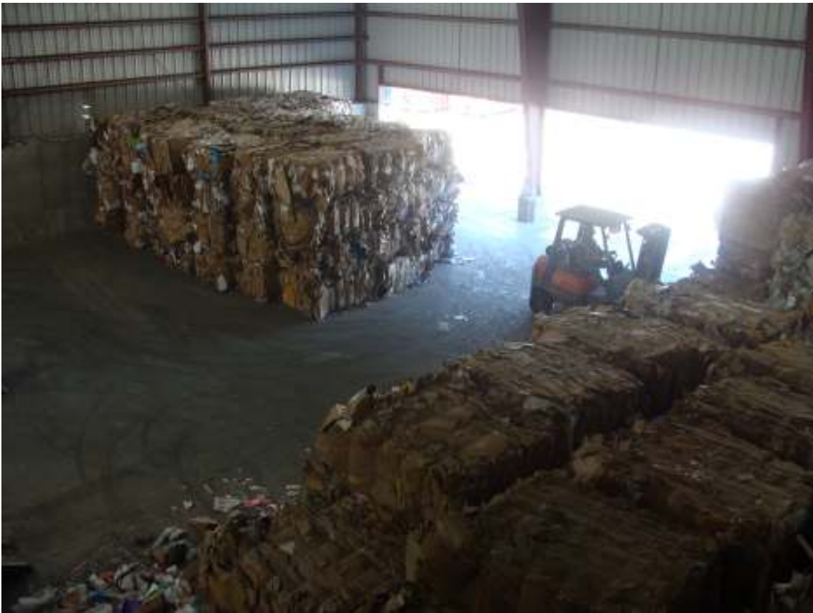
Picture 6: Finally, the separated materials are baled for resale and reprocessing into new paper and manufactured goods.
