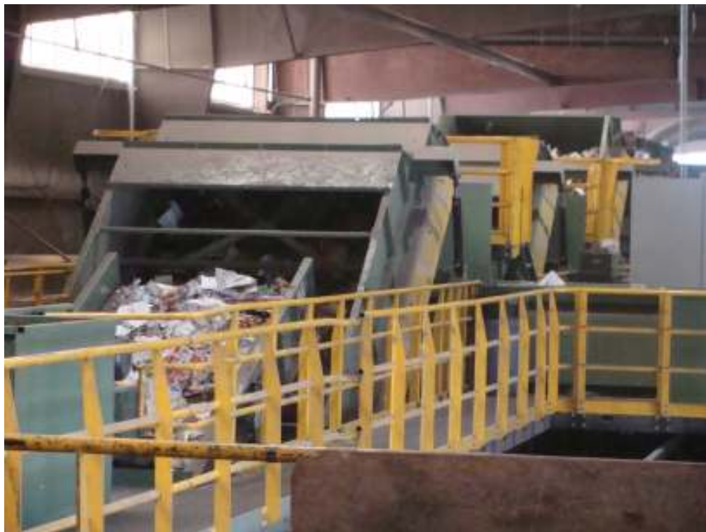
Picture 3: A series of three inclined screens separate materials by density. Different types of plastics are sorted out by optical scanners, and metals such as aluminum cans are sorted by eddy current sorters.
