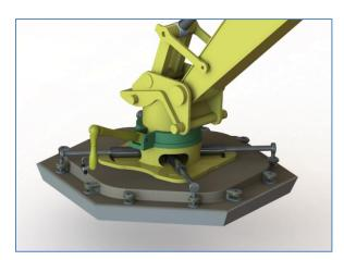
The assembly of the structure will be accomplished by a robotic excavator with a specialized end affecter consisting of set of hydraulic grippers and a robotic welding arm. It will lift the panels by inserting the gripper ends into the anchor supports and extending the hydraulic arms, creating tension within the panel. Once the tile is lifted and aligned in place, the laser welding arm can travers the perimeter, welding the adjacent panels. Initially we were
