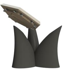
brittle and weak in tension. To overcome this, the supports created with this material will be and minimal build angles and only loaded in compression. Below the basalt supporting structure can be seen, as well as a Tile with a positioning feature molded in place. This is only required on the lower tiles of the small volumes.
