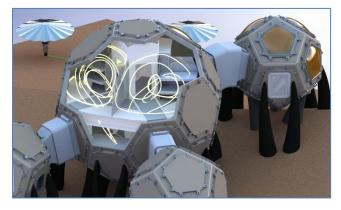
Additionally, detailed below, are the individual heater/CO2 Scrubbing units for the smaller volumes. Though the primary heating and oxygen generation is to take place in the lower level of the primary volume, it is important to be able to heat the volumes and scrub CO2 independently in the event of a separation of the volumes due to unscheduled depressurization of the habitat.
