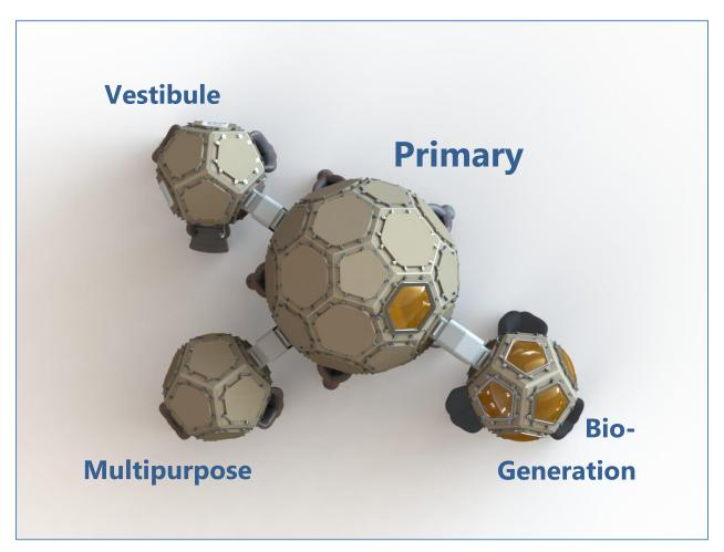
The Habitat consists of 4 volumes as shown above. They each provide unique functional environment for a year-long mission to Mars. All the individual cells have an independent electrical supply for redundancy. In addition, there are emergency air tanks in each of the small cells to supply fresh air for a period in case of a breach in the seals or a catastrophic failure of a volume.
